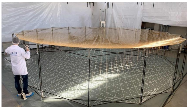
Figure 2: European Large Deployable Reflector fully deployed
