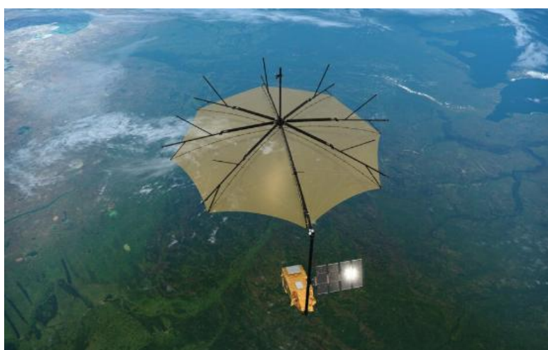
Figure 1: ESA Biomass satellite over forest with 12m mesh reflector unfurled 1
